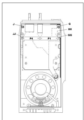
Figure 10 - Keypad Flex And LCD Board Access
